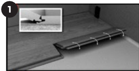
STEP 1: Lock long edge of plank by inserting tongue into groove at an angle and drop in place.
