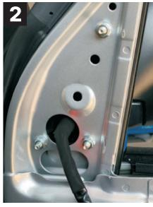
Hold the mirror in line with the bolt hole, and you will need to use the three supplied nuts to secure the bolts. Place all pre-fixed studs through the door and start the top bolt off and secure about half way up the thread. Once finished, double check that the rubber surround on the door isn't stuck under the mirror base and the rubber seal sits flush against the mirror and door frame. Next, tighten the 3 bolts until they are securely tightened.
