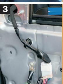
The mirrors are supplied with a plug and play loom that will directly plug into the original one you have just disconnected. Ensure this clicks firmly into place.
