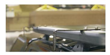
(2) If you mount your shower tent to the mesh of a roof rack, the L brackets go on top of the mesh and the sandwich plates underneath. Use the long bolts to sandwich them together.
