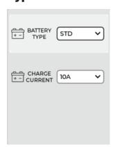
Before charging, select the correct battery type and charging rate. The interface provides options for four battery types: 12V/24V STD (Standard Lead-Acid), 12V/24V AGM (Absorbed Glass Mat), 12V/24V CAL, and 12V LFP (4-cell LiFePO4). Users can also choose from four charging rates: 10A, 20A, 30A, and 40A. Press the UP or DOWN button to select, then press the ENTER button to confirm.
