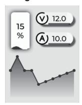
During charging, the interface displays the battery's charging percentage, voltage, current, and current curve. To exit charging, press the RETURN button.
