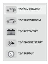
The home interface features five key functions of the product: 12V/24V Charge, 12V Showroom, 12V Recovery, 12V Engine Start, and 12V Supply, all displayed for easy access. Users can navigate the interface using the UP and DOWN buttons to scroll through the options and confirm their selections with the ENTER button.
