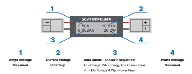
Data Queue - When power is supplied to the watt meter, the unit will start recording data. To reset the Data Queue to zero, simply disconnect the watt meter from power, wait 30 seconds and reconnect.
