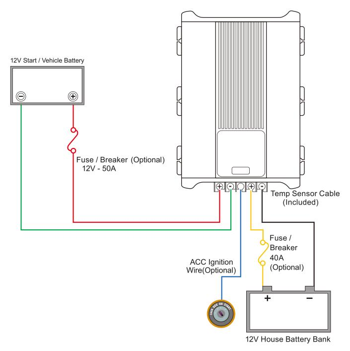
NOTE: First connect the ACC line to the ignition of your vehicle. Then turn your key to the ACC position when engine starts, which will be detected by the DC-DC charger. And your auxiliary battery will be charged via the main battery.
