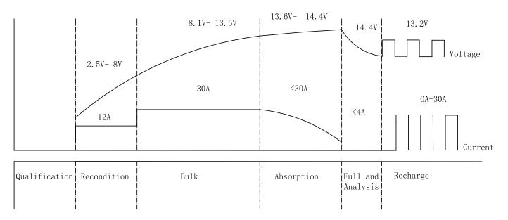
Charging algorithm will change according to battery type.
