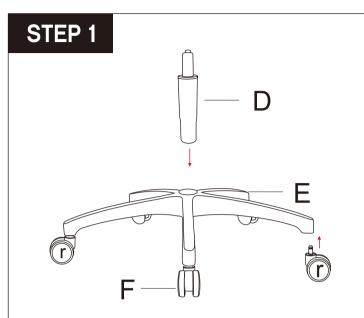
Press the Casters (F) into the holes at the end of each leg of the Base (E).
