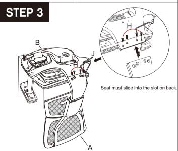
Please be careful to use the correct Back Bolts (H). Attach the Backrest (A) to the Seat Cushion (B) using 4 Back Bolts (H).
