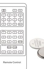
Tips: By default, the remote control is not equipped with batteries, due to the safety requirements of some express companies. Install CR2025 cell before use.
