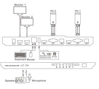
Note: Both HDMI and VGA cables should be connected to PC, if only connect HDMI or VGA cable, then the dual monitor function would not work properly.
