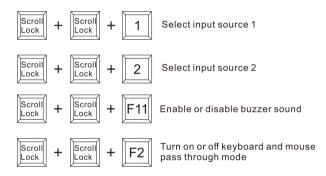
Note: For the best compatibility, it is better to turn on keyboard and mouse pass through mode. In this mode, the keyboard and mouse are dynamically mapped to computer, so you are able to use special keyboard and mouse that with multimedia keys or other customized
