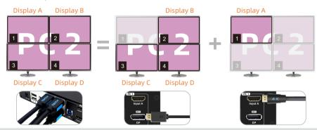
**Tips:** If a device that doesn't support MST is connected, the display will only show on output A or show three duplicated screens. The specific situation depends on the device.
