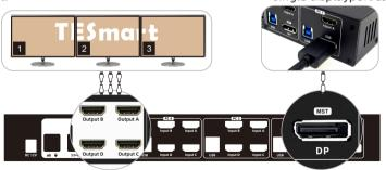
Tips: 1. Limited by bandwidth, the output resolution via MST supports a maximum display of two 4K60Hz 4:4:4 and one 4K30Hz 4:4:4 displays.
