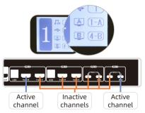
We have set up a switch mode for retaining the HPD signal, which can be enabled or disabled according to your needs. Use keyboard hot key to enable or disable the HPD retention mode. HPD retention mode is enabled by default. You can use keyboard hotkey command [Right-Ctrl] + [Right-Ctrl] + [F4] to switch states.
