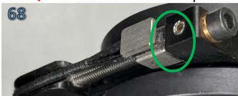
3. Visually inspect the bowstring spreader located at the front of the crossbow to ensure it is aligned at a 90-degree angle with respect to the frame. You may use a small measuring square or the corner of a piece of binder paper to check for proper alignment as shown in photo #69.
