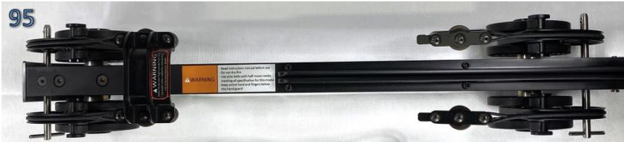
7. The new bowstring may now be installed. Follow the stringing diagram and instruction in the String Change section to complete the installation process.
