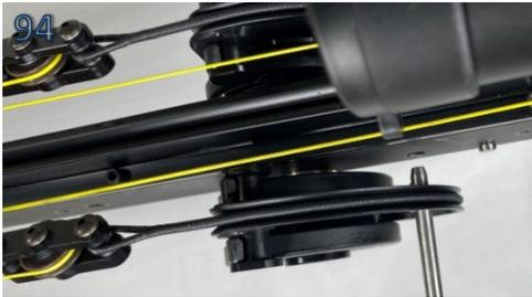
6. After both pins are secured in the front and rear cam and frame ports, the cocking winch may be removed and the tuning string can be removed, as shown in photo #95.
