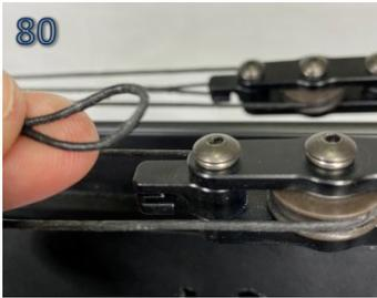
12. Take care to ensure the pulley cables stay within the cam grooves while unwrapping the old bowstring from the pulleys.
