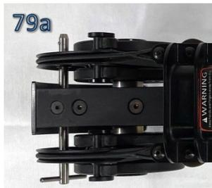
9. On the rear cams, rotate the cam tensioning screws counter-clockwise on each cam, alternating between each cam to ensure the tension is balanced between each of the rear cams until all the rear ports are in alignment and then insert the other pin through the rear ports. **STOP rotating the tensioning screw when the anchor just makes contacts with the cam**, as further counter-clockwise rotations risk releasing the cable anchor, resulting in serious injury and property damage.
