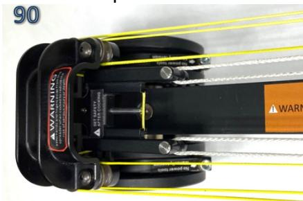
3. **STOP** and visually inspect to ensure the tensioning string is within all pulley grooves. Slowly tension the cocking winch and continue inspect the pulleys to ensure the tuning string stays inside all of the pulley grooves, as shown in photo #91 and #92. They tend to slip out until the pulleys have become level.
