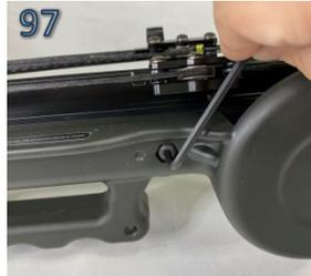
2. Reposition crossbow on its side with the fasteners heads that secure the plastic covering facing upwards. Using a 3/16" hex manual key or ratchet tool, begin removing the (two) 8-32 x 1/2" flathead screws on the front of the crossbow, as shown in photo #98.
