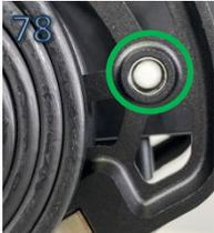
7. If the FRONT cam ports are not yet aligned with the front frame ports, un-tension the REAR cam tensioning screws, alternating a few counter-clockwise rotations on each rear cam tensioning screw until the point that the FRONT cam ports are aligned to the front frame port.
