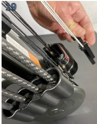
4. Insert the cocking sled into the spreader and over the top of the bowstring center serving and ensuring both of the hooks engage the bowstring throughout the entire tensioning process, as in photo #20.
