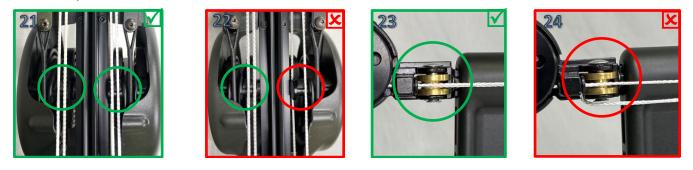
**6.** Once the winch cables are clear and you are certain both hooks of the cocking sled are engaged on the bowstring, you may continue to smoothly crank the winch handle until the point that it is engaged into the
