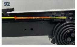
**4.** Continue to slowly add tension to position the front cam port in alignment with the frame. When the ports are in neat alignment, you make take your hand off the cocking winch and test the pin's fit in the ports. If the fit is tight, advance the cocking winch crank by ¼ turn and test the pin fit again. The ports in the cam and frame are designed to allow the pin to easily slide in, as shown in photo **#93.**
