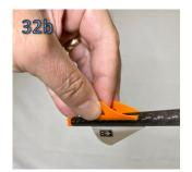
2. Point the tip of the arrow through the space within the spreader and picture, as shown in photo #33.
