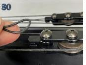
**12.** Take care to ensure the pulley cables stay within the cam grooves while unwraping the old bowstring from the pulleys.
