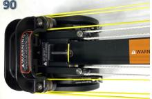
3. • STOP and visually inspect to ensure the tensioning string is within all pulley grooves. Slowly tension the cocking winch and continue inspect the pulleys to ensure the tuning string stays inside all of the pulley grooves, as shown in photo #91 and #92. They tend to slip out until the pulleys have become level.
