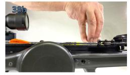
**3.** Grasp the arrow by the fletching vanes to remove the arrow, as shown in photo **#39**, and secure the it in your quiver.
