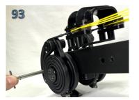
5. After the front pin Is secured through both cams and the frame ports, slowly turn the cocking winch handle to align the rear cam ports with the frame port. Again, test the pin fit into the cam and frame ports until it easily slides in, as show in photo **#94**.
