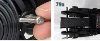
9. On the rear cams, rotate the cam tensioning screws counter-clockwise on each cam, alternating between each cam to ensure the tension is balanaced between each of the rear cams until the all the rear ports are in
