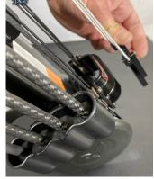
**4.** Insert the cocking sled into the spreader and over the top of the bowstring center serving and ensuring both of the hooks engage the bowstring throughout the entire tensioning process, as in photo **#20**.
