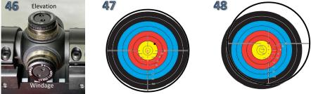
3. After achieving an approximate zero at 10 yards, move back to a measured 20 yards and continue adjusting the turrets until the top cross of the reticle and the point of impact are the same. Use the top crosshair labeled 20 yds in your reticle, as shown in photo **#49.** At this range, each click equals 1 /10 of an inch (10 clicks to move the impact 1 inch). When you are happy with the 20 yard zero, replace the turret covers.
