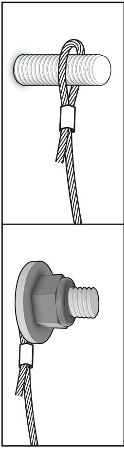
Hook loop-end of tether around an anchor and secure as shown.
