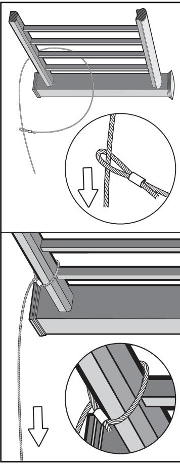
Loop tether through a secure structure and feed through loop-end as shown.
