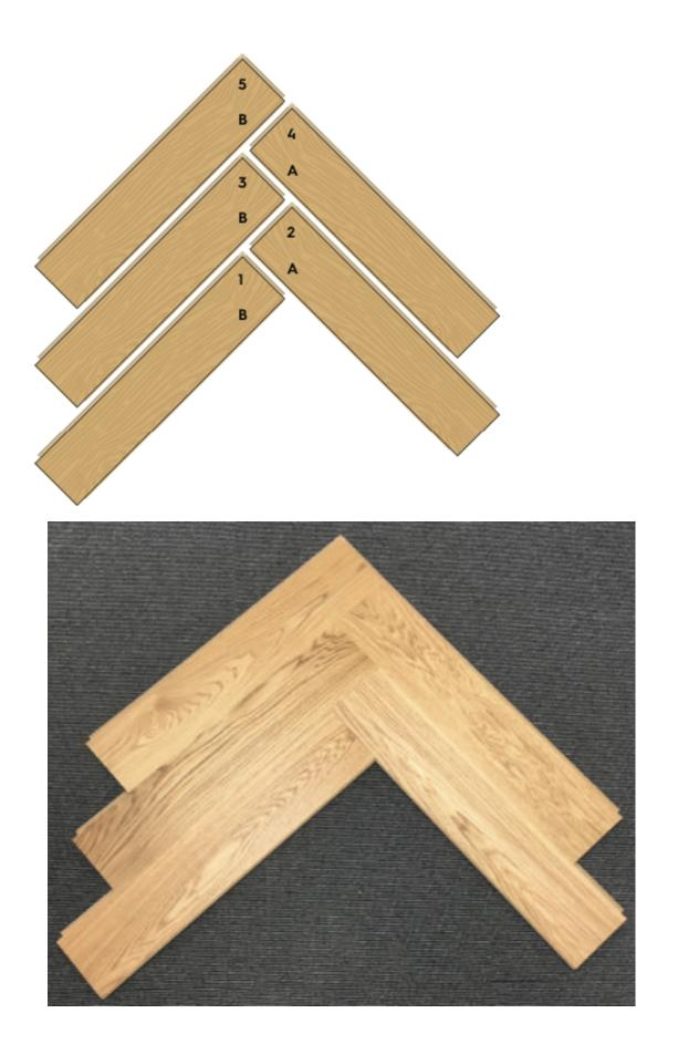
Install the boards precisely and in the order indicated by the numbers on the boards. Carefully check the joints between the planks after every plank which is added. No protruding edge should be felt.
