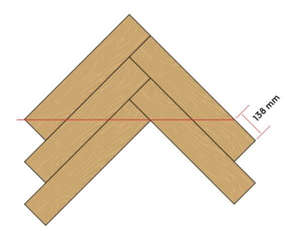
In case you have calculated and built an uneven number of triangles, leave the outer two triangles aside. In case that you have built an even number of triangles, lay one aside. Lay out the middle triangles with their long side towards the starting wall. Make sure the underlayment is installed beforehand and the installation line remains visible.
