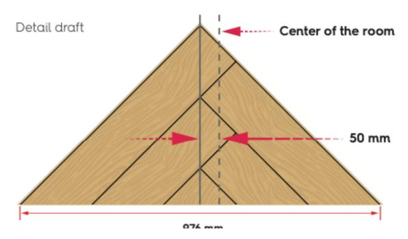
Use expansion wedges for the expansion gap. Make sure the top of the centered triangle is on the installation line (50 mm left from the center). Check the straightness of the starting wall. If it is not perpendicular to the center line, the starting triangles
