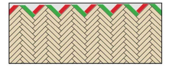
it to close the open gaps to the finishing wall. Use the leftover from planks 1, 2, etc. consecutively and cut to size if necessary.
