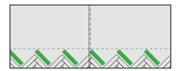
Now install B-planks and cut the most right piece to size.
