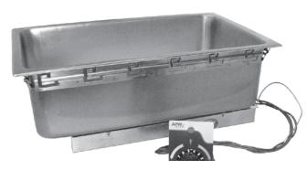
APW Wyott uninsulated drop-in hot food wells are supplied with a UL Listed approved electrical kit includes an electrical conduit, control box and bezel or a UL Registered kit with thermostatic controls, pilot light and a 36" capillary.
