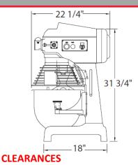
The top and bottom of the mixer must remain open and unobstructed. A clearance of at least 6" (152mm)
