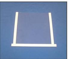
Using the four clamps supplied, clamp each of the four outside corners of the gel sandwich assembly. If desired, using the bottom spacer is not required. Simply, align side spacers with bottom of glass plates and tape bottom edge of glass plate assembly with casting tape (CTP-125). When taping bottom of glass plate assembly make sure to fold tape up around the corners approximately 1 inch.
