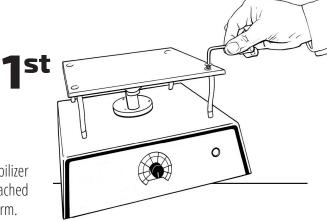
First, remove the four screws attaching The Belly Dancer® platform to the flexible stabilizer legs at each corner. Use the provided hex wrench enclosed in the kit, save the detached screws for later use. Do NOT remove threaded standoffs from bottom of acrylic platform.
