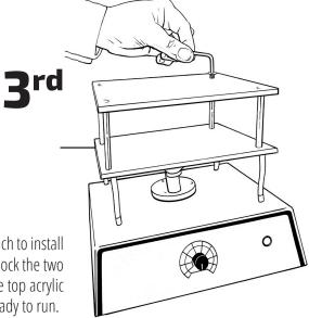
Finally. align the new 2nd story platform with the four spacer legs. Use the provided hex wrench to install the screws, previously removed in step 1. Tighten all four screws, in all four corners, this will lock the two platforms together. Replace the bottom silicone mat, and place the new supplied mat on the top acrylic platform. Reconnect your Belly Dancer® unit to an electrical power source and you will be ready to run.
