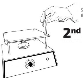
Second, install the aluminum spacing rods by threading them into the existing standoffs (thru the acrylic platform) in which the screws were just removed. Hand-tight is fine for these items.
