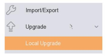
You require the Firmware file on a USB Storage Device, connected to the recorder. In this menu you should see the Firmware File. It should be called Digicap.dav. Firmware Files downloaded from Hikvision's Portal come in a Zipped file format, and the actual firmware will need to be extracted to the USB Storage Device prior to Upgrade, as the recorder cannot read the Zipped format.
