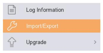
This allows us to export a Config file with all our devices settings to a connected USB Storage Device or Import a Config File from another device to this device from a USB Storage Device.
