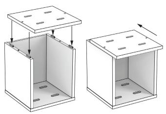
Place top panel onto channel locks and slide top into position.
