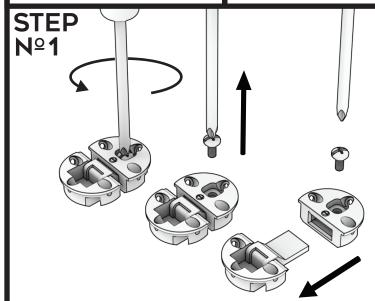
Unscrew bolt and disassemble flap hinge.
