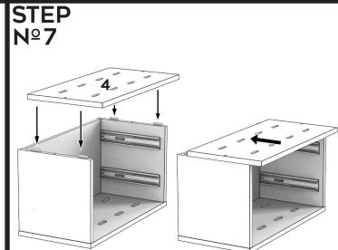
Place top panel onto channel locks and slide top into position.
