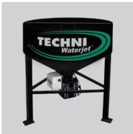
The hinged lid on the hopper system allows easy access to inspect and fill at any time, without the need to de-pressurize. The clear pump chamber allows a quick visual to ensure abrasive is present and flowing correctly. Here is where the abrasive is pressurized, allowing the hopper lid to be opened at any time.
