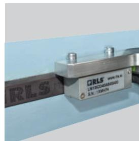
The Linear Scale Feedback is what makes the highest tolerances possible. By mapping the entire cutting area with a laser-calibrated digital interferometer, the motion system can deliver positional accuracy of 0.05 mm (0.002"). Repeatability of motion is increased to 0.025 mm (0.001").
