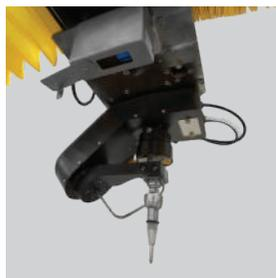
The Laser performs a precise mapping of the workpiece to increase the accuracy of the cut. It's able to map pierce points, the full sheet, and paths, as well as find origin and edges of the sheet.
