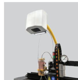
Tech-Vision Camera allows to effectively match parts that will be mounted close together, helping the operator to perform book and waterfall matching panels.
