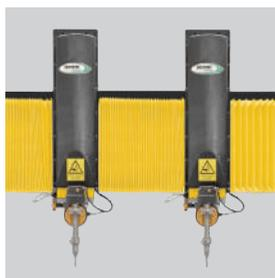
Twin cutting heads increase the productivity. The machine will run the program once but twice the amount of parts are being cut. Pump power is a key decision variable when considering this option.
