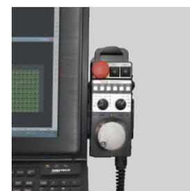
The MPG gives full jogging control in X-Y & Z allowing to manually wind forward or backward through a cutting path. This enables the operator to find the exact point from which to restart cutting after a stoppage, or to simply locate a pre-cut part.
