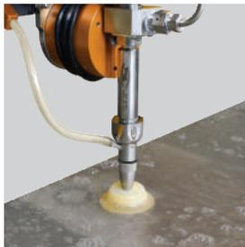
Water Raise & Lower at the push of a button for quieter, cleaner and safer submerged cutting; our tanks include air-tight welds of an air chamber which uses regular shop air pressure to raise or lower the water level. No moving parts are required, an on/off solenoid valve allows water level adjustment within a few seconds.
