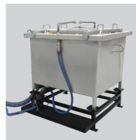
The GRS collects used abrasive accumulated in the bottom of the Waterjet tank. The abrasive is pumped to the GRS where it settles into a bag while the water is returned to the waterjet tank.
