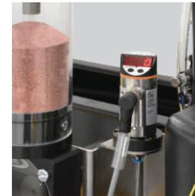
With our new variable abrasive feeder, garnet supply to the cutting head is automatically adjusted by the software, e.g. during low pressure piercing. In addition, the Tech-Sense Monitoring System enables truly unattended operation. After an interruption, the cutting program can be easily resumed.
