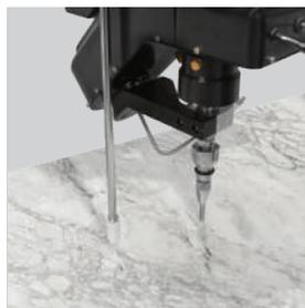
Touch-Probe performs terrain mapping by touching the surface of the slab. This allows the cutting head to automatically adjust its standoff.
