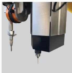
Drilling Head avoid delamination or cracking of materials such as composites and laminated by drilling a small hole instead of using the cutting head for the piercing process.
