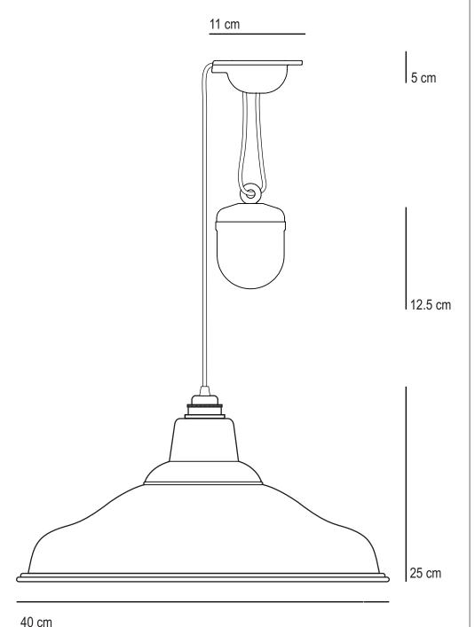
Cable length may be shortened upon installation. This will reduce both maximum & minimum drop and reduce the range of movement.
