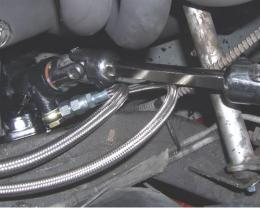
4. When connecting your pressure and return lines, your pressure line goes from the lower port on the rack housing to the banjo fitting on the pump. The return line goes from the top port on the housing to the plastic reservoir on the pump.
