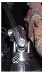
9. U-joint orientation is very important. When bolting intermediate shaft assembly into place. Install the joints 90 Degrees off of each other. This is important, as it will reduce "BUMP", the hard points of rotation in the steering. With the shaft and u-joints connected tighten the setscrew on the top u-joint and drill through the shaft and column insert using the u-joint as a guide. Note: Make sure steering wheel is locked in the straight position and the rack is still centered.
