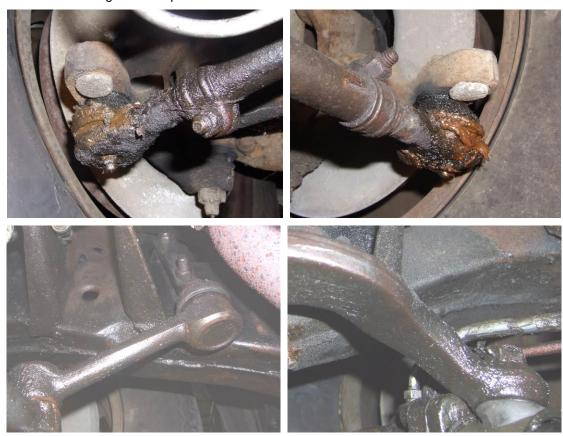
3. If your car was equipped with power steering, you will have a bracket mounted on the bottom of the driver's side frame. This bracket holds the power assist cylinder. You can now remove this bracket.
