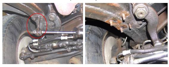
4. Remove stock steering linkage from vehicle.
