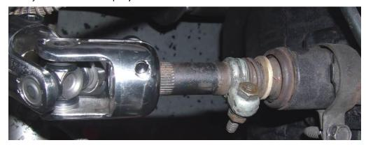
9. With upper u-joint on column with pinch bolt running across the flat on the shaft. Raise rack and pinion assembly up in between the frame rails. Line lower u-joint up with the splines on the pinion. Slide u-joint onto pinion.
