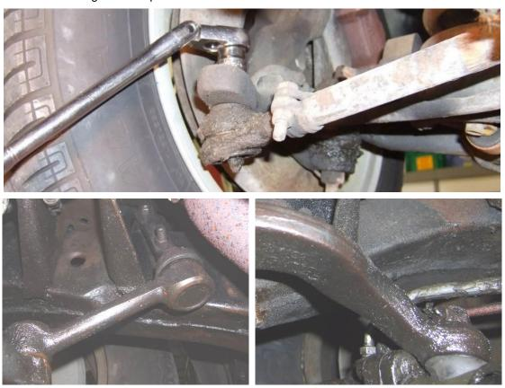
3. If your car was equipped with power steering, you may have a bracket mounted on the bottom of the driver's side frame. This bracket held the power assist cylinder. You can now remove this bracket.
