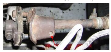
7. From above vehicle, measure 2 3/8" from the end of the steering column shaft and make a mark on shaft. Trim end of shaft off at 2 3/8" mark.
