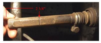
8. With rack centered in vehicle and steering wheel locked in the straight position, install intermediate shaft assembly. Note: Inside of top u-joint should be flush with end of column shaft.
