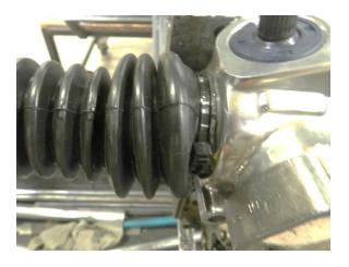
9. With a sharp blade carefully cut around the outer edge of the O-ring against the end cap to give a nice clean look.
