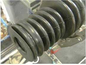
8. Use the new zip-tie around the inside boot lip. Tighten it down and cut.
