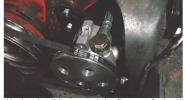
15. With power steering pump bolted in place, install the correct v-belt to fit your application. You will have to measure the length of belt you need. It is best to get a few sizes and then return the ones you don't use to limit trips.
