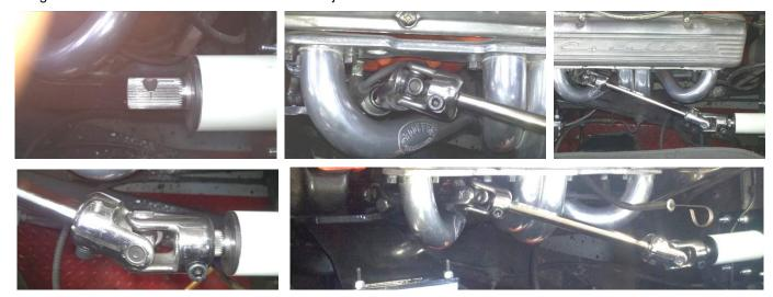
13. Make sure entire shaft assembly is routed without interference. Tighten u-joints and the shaft support bracket. Make sure the jam nut on the hiem joint is tight as well.
