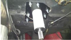
10. With column in correct location in vehicle, tighten the upper clamp bolts and the supplied tube clamp on the inner firewall plate. At this point you can install the steering wheel as well.
