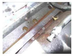
10. Remove all the bolts from the lower steering arm assembly, as well as the tie rod ends from the spindles and the steering linkage to the gearbox.
