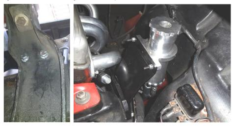
8. Place (Ididit) column in place with inboard firewall plate over steering column tube (it won't fit after the column is thru the firewall). Begin by installing the column clamp under the dash, directly behind where the steering wheel will be. Mount steering column in factory location (with the bell of the column approx 1/8" away from making contact with the dash).
