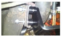
5. With kit bolted up in chassis, make sure the bracket is perpendicular to the bottom of the frame. Notice that on the mounting bracket, there are two round holes and two slots. The slots allow this adjustment. When bracket is set to correct angle (90 Degrees perpendicular to bottom of chassis) Tighten bracket bolts down to the suggested: 36 ft lbs.
