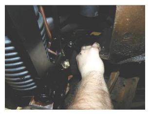
19. Install the outer tie rod ends and tighten lock nut on steering arm to 45 ft. lbs. Adjust the toe by eye so you can drive to an alignment shop. This is done by turning the inner end. You do not have to take off outer end to adjust. Tighten jam nut once toe is set. Screw in Zerk fitting and grease.
