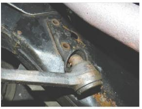
4. Remove tie rods from spindles.
