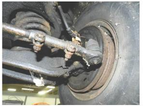
3. Disconnect the center link, power cylinder, idler arm.
