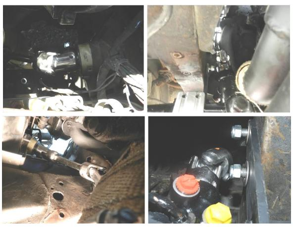
9. You can now torque the mounting bolts for your rack to 65 ft. lbs. Then torque the u-joint bolts to 40ft lbs.
