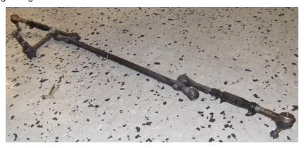
4. With stock steering removed, thread supplied 11/16-18 LH jam nuts onto threads. Run jam nuts all the way till they are at the ends of the threads. At this point thread the supplied ends into new tie rod adjusting bars.
