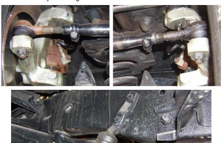
2. Remove the pinch bolt from the input shaft on the steering box. This will allow for the gearbox to be completely removed after removing the three bolts holding it to the frame.
