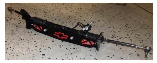
5. Now to install your new kit. With supplied hardware (2: ½-13 bolts and 2: 3/8-16 bolts). Bolt new R&P kit up into frame. Note: ½" bolts are used in driver's side (Holes may need to be reamed) and 3/8" bolts are for passenger side.
