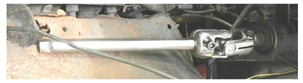
5. Slide support bearing with bracket up shaft. Line brackets up with holes on frame as pictured and bolt bracket down.
