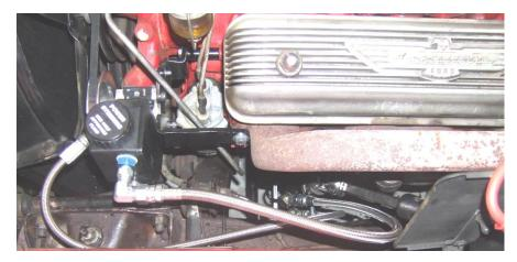
Note: There is a tube inside the pump reservoir, on the return side, which may make the reservoir cap a little difficult to reinstall.
