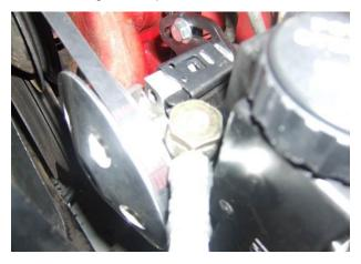
13. From under the car, you are now ready to install the power steering pressure and return line. The pressure line has two straight ends on it and is smaller in diameter. The pressure line has to be connected to the lower port on the rack and pinion assembly and goes to the banjo fitting on the top of the power steering pump.
