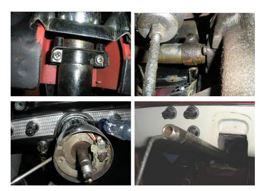
3. Next remove the steering box bolts on the driver side of the frame and remove the gearbox entirely with the shaft. Next you will need to modify your column tube. First measure up from the bottom of the column tube that was connected to the gearbox 5.5" and cut off that portion using a tube cutter or band saw. Make sure to do this accurately and squarely.
