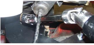
10. Tighten the wheel nut to 40 ft. lbs. From under the car, you can connect your outer tie rod ends and torque them to 65 ft. lbs. You can now tighten the main mounting bracket and shaft support bracket to 65 ft. lbs. Note that the shaft support is slotted on one end which allows it to rotate up and down a little for column angle and u-joint angle.
