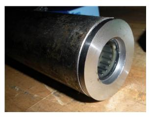
6. Next install the new upper column bearing. Install this in the same manner as the lower bearing and install the original snap ring to hold it in place.
