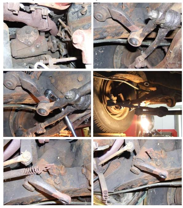
4. Remove the 2 retaining bolts on the idler arm assembly. Remove the idler arm and the rest of the steering linkage.
