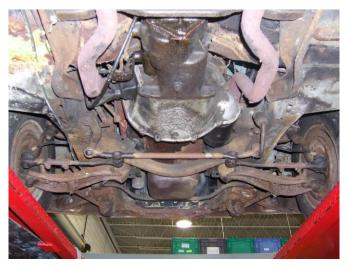
2. Remove front tires. Remove outer tie rod ends, cotter pins, and retaining nuts. Remove outer ends from spindle.
