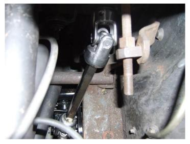
16. Last, we need to install the pump. The bracket and pump were shipped assembled you need to remove your old pump and bracket assembly if equipped. Install the main mount bracket and pump in place using the 2 standoffs and longer 5/16" bolts. You must remove the 2 water pump/ timing cover bolts and install the bracket and standoffs in their place with the longer bolts.
