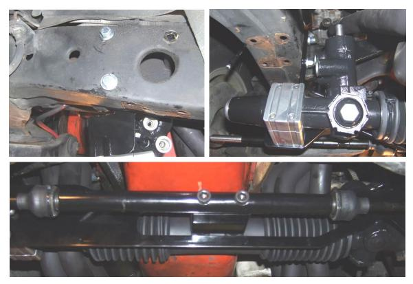
3. Thread lock nuts and tie rod ends onto the inner tie rods.
