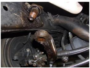
3. Remove the steering linkage from the car. If the car has power steering remove the lines from the assist unit and remove it with the linkage.
