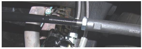
16. From under the car, you can install the pressure and return line in place. The larger hose is the return line and goes on the top port closest to the pinion. The smaller hose is the pressure line and goes on the lowest port of the rack. Route the lines up the frame to the new pump in the shortest route. You will need to install the two banjo fittings first on the rack. Torque to 18 ft lbs and only torque down once or fittings will leak.
