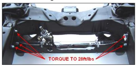
Line up the holes in the mounting brackets to the holes in the frame, where the steering box and idler arm were. Bolt brackets onto the frame, using mounting hardware kit **#620340**. Nuts to the inside of the frame, bolt the brackets into the frame with 28 ft/lbs of torque (see illustration Above).
