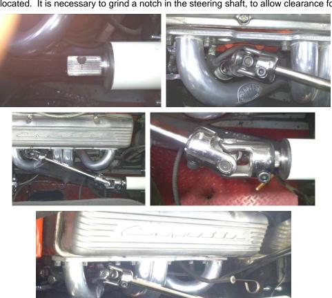
13. Make sure entire shaft assembly is routed without interference. Tighten u-joints and the shaft support bracket. Make sure the jam nut on the hiem joint is tight as well. Tighten rack bracket bolts down to the suggested: 36 ft lbs.
