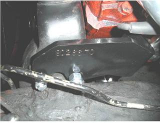
3. Place supplied (Ididit) column in place with inboard firewall plate over steering column tube (it wont fit after the column is thru the firewall). Begin by installing the column clamp under the dash, directly behind the where the steering wheel will be.
