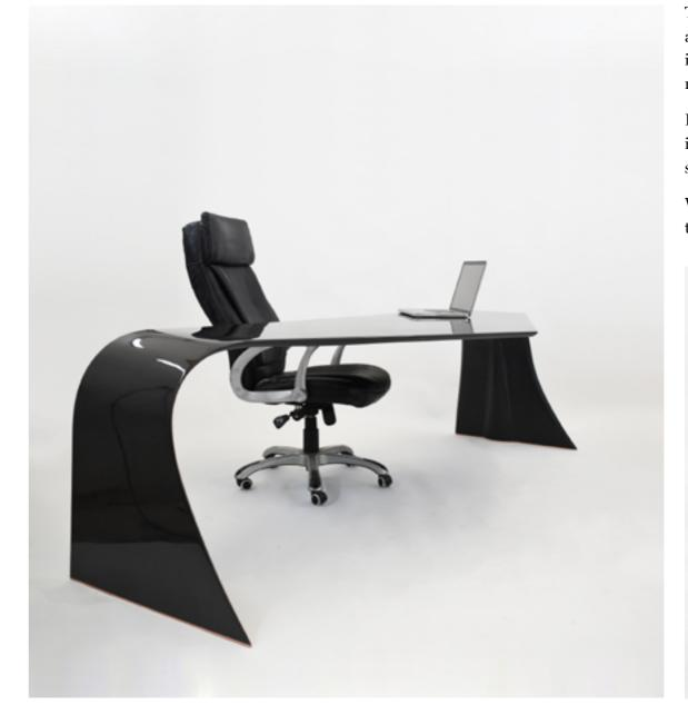
To achieve this the Vulcan desk is manufactured using a core of aerospace grade carbon up to 18 layers thick. Oriented in a quasi-isotropic pattern in key areas to achieve the necessary torsional rigidity and dampening required.
