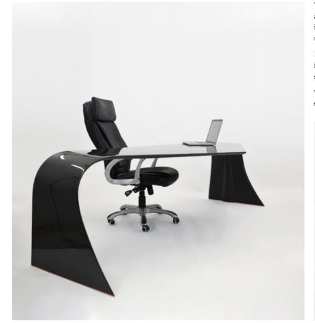
To achieve this the Vulcan desk is manufactured using a core of aerospace grade carbon up to 18 layers thick. Oriented in a quasi-isotropic pattern in key areas to achieve the necessary torsional rigidity and dampening required.
