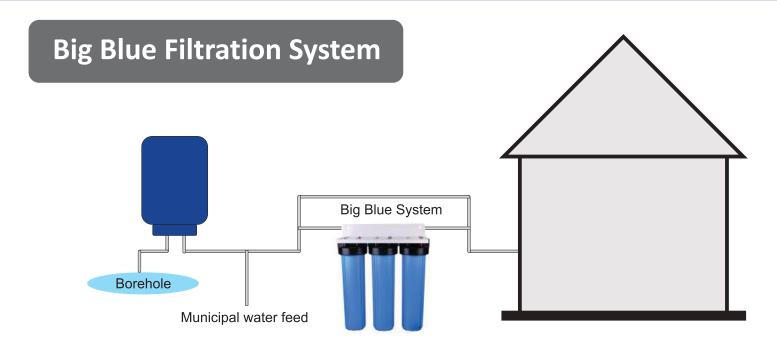
Flow rate of a 20"Big Blue System: 20-25L/min Filter combination dependent
