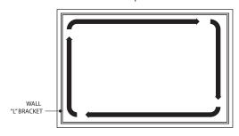
3. Fasten every 16" - 24". The corners can either be mitered to 45° or butt jointed.
