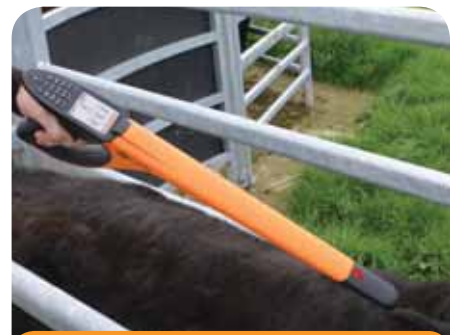
The HR5 screen clearly displays the visual ID and count of animals in the session.
