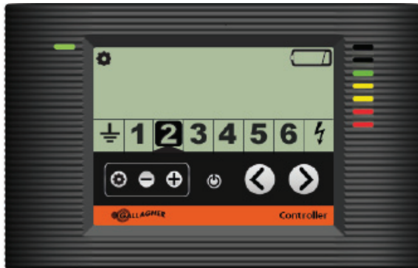
Controller showing zone 2 with a low battery
