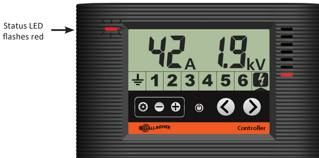
Controller showing the energizer in output alarm
