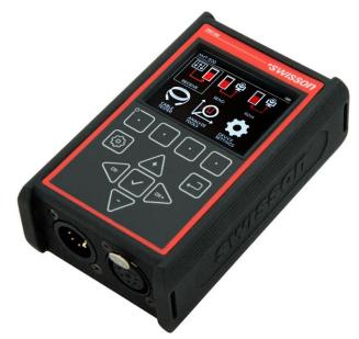
well as RJ-45 cable automatically. Thanks to the *cable test dongle*, even installed cables can be easily tested.
