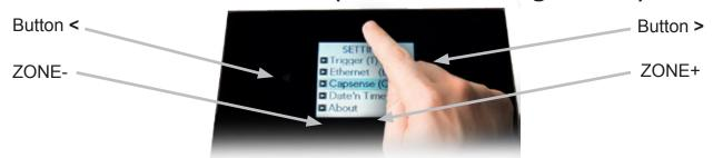
To access the settings menu, hold the on/off button for 3 seconds.
