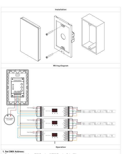
The controller can control many DMX Decoders, All DMX Decoders Set as 001 Note: one DMX Decoder has 4 channels, so take 4 DMX Addresses 001, 002, 003, 004
