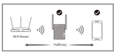
For optimal Wi-Fi signal, please install the Wi-Fi extender around 2.5 feet or more away from your floor. Installing it too close to your floor may lower extended Wi-Fi signal.
