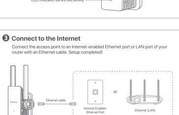
\* The LED indicator lighting solid blue indicates a successful Internet connection. Otherwise, refer to Q2 in FAQ to reset this access point and try again.
